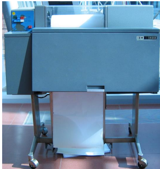
A Card punch machine and IBM 1403 line printer, the classic line printer of the mainframe era.
